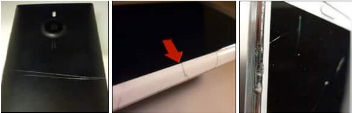
Cracked casing or frame
